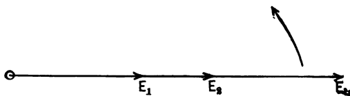
FIG. 60. The voltage wave E_1 has completed two more cycles since Fig. 59, and is \frac{1}{2} cycle further ahead of E_2 . This causes E_2 and E_1 to be momentarily in phase and the resulting voltage E_L is a maximum.
